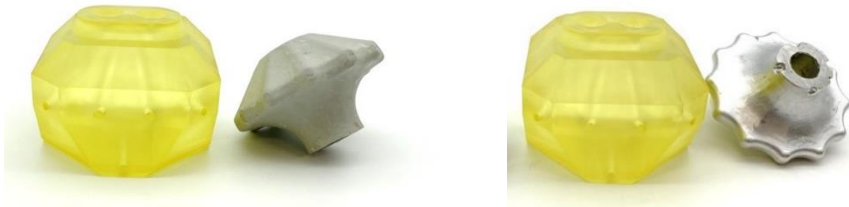
Figure 1: Examples of printed mold and final object, shown for a glass fiber-filled 2K epoxide (left) and the 'Fieldsche Metal' as low-melting allow (right).
